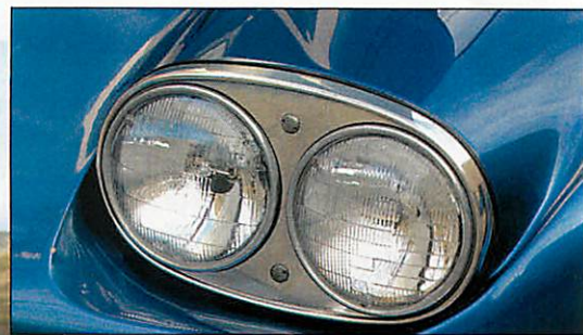
Earlier models had single-piece Cibie headlamps; 400GT 2+2s all had quad sealed beams
