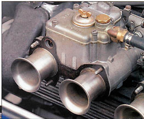
Seven grand is on the high side for a street car V-8 in the '60s, but this V-12 pulls clear through. Six twin-throat Webers mean that every cylinder has its own carb throat.
