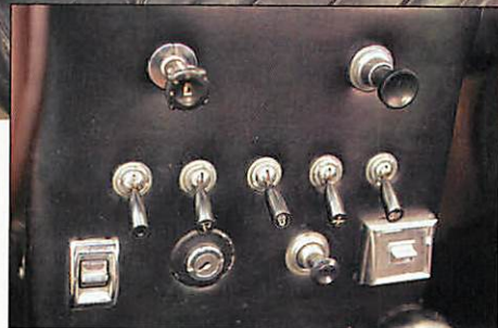
Unlabeled toggle switches look cool, but the backing panel is shaky
